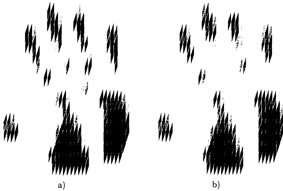
Figure 3.18: Unsmoothed a) and diffused b) proximity images of a flattened right hand rotated counter-clockwise about 30^\circ .
