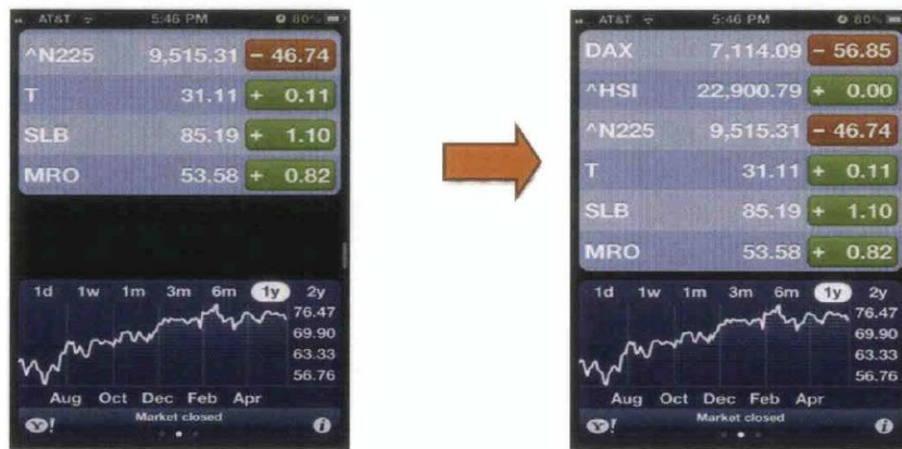
(Bounce-Back Scrolling in iPhone Stock Application When Finger Is Removed From Touch Screen.)
