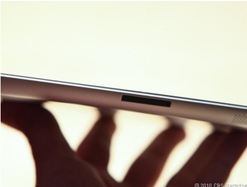
**The height and width may look similar, but in terms of thickness, the iPad has done some dieting, shrinking from 13.4mm thick on the original model to 8.8mm thick for the iPad 2. It's thinner, even, than the iPhone 4.**
