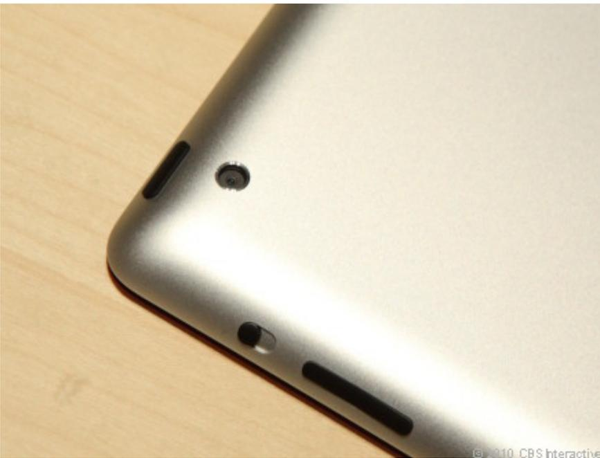
**The iPad 2 boasts two cameras; the original iPad doesn't even have one. The rear-facing camera, pictured here, supports 720p video capture.**
