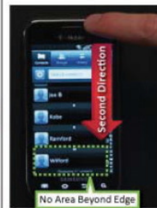
Figure 4: When finger is lifted, document is moved in second direction to display “fourth portion” with no “area beyond edge”
