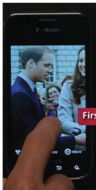
Figure 2: Displaying “second portion” by moving document in first direction in response to finger movement on touch screen
