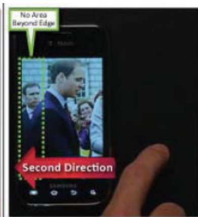
Figure 4: When finger is lifted, document is moved in second direction to display "fourth portion" with no "area beyond edge"
