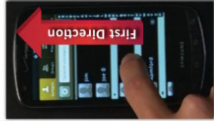
Figure 6: Displaying "second portion" by moving in first direction in response to finger movement
