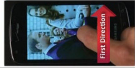
Figure 2: Displaying "second portion" by moving in first direction in response to finger movement
