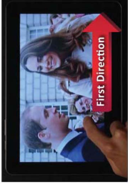
Figure 2: Displaying “second portion” by moving document in first direction in response to finger movement on touch screen
