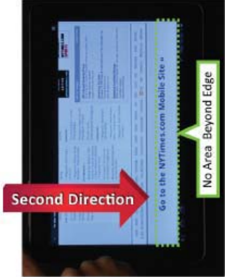
Figure 4: When finger is lifted, document is moved in second direction to display “fourth portion” with no “area beyond edge”
