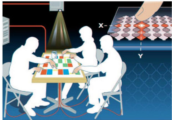
Figure 1: Prototypical DiamondTouch setup: front-projection onto a tabletop surface.
