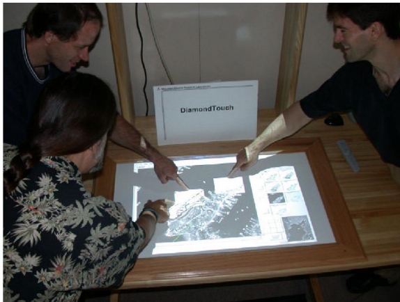
Figure 4: An overview shot of DiamondTouch running DTMap, a multi-user, layered information, map application.
