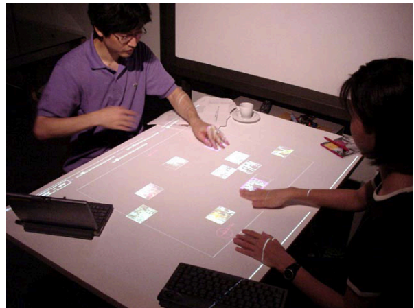
Figure 1: An interactive surface system based on the SmartSkin sensor.
