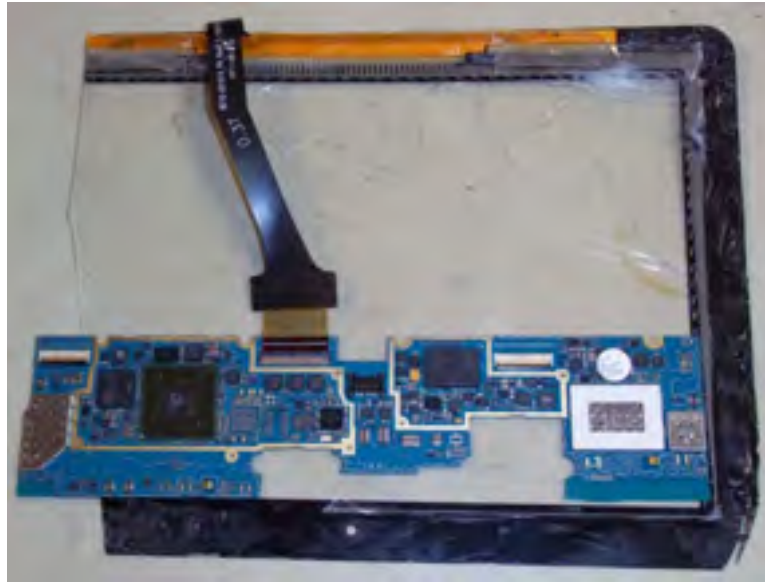
Figure. Camera image of the Galaxy Tab 10.1 touch screen, connective flexboard, and circuit board. See Exhibit C-64.
