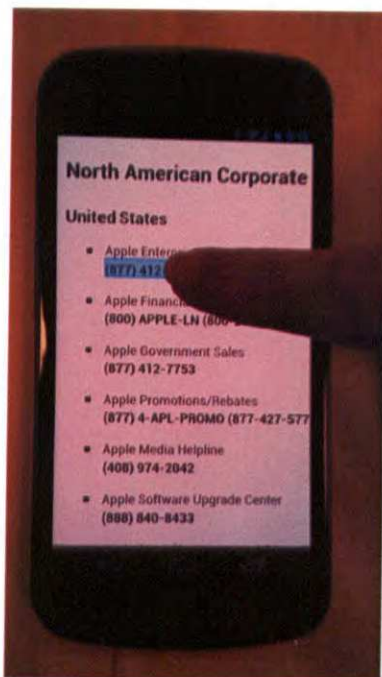
23 24 Browser on Samsung Galaxy Nexus – phone number is highlighted when a user begins a long-press on a detected 25 phone number in a webpage
