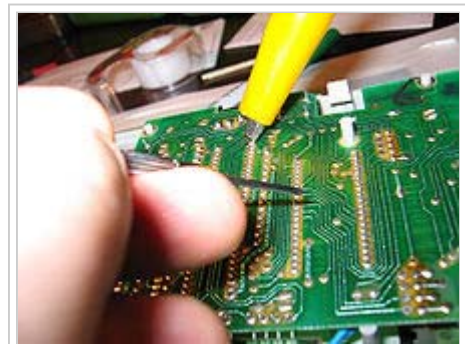
A DIY musician probes the circuit board of a synthesizer for "bends" using a jeweler's screwdriver and alligator clips
