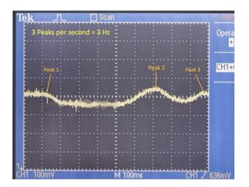
(<u>Id.</u> ¶ 213.) Dr. Welch measures the signal's frequency by counting the peaks ("Peak 1," "Peak 2," and "Peak 3") and dividing by the duration of the recording (1 second) to yield a frequency of 3 Hz. Because 3 Hz is less than 20 Hz, Dr. Welch concludes that this signal does not meet the definition of an "input signal." This approach inherently yields a single number regardless of whether the signal is made up of one or multiple frequencies.
