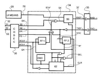
('730 patent, Fig. 4A.) "Block 34" of this figure, which corresponds to the "framer," is denoted by the dashed line. Other components of this figure that have been the subject of expert testimony are block 50, which is a "data selector"; block 62, a "clock generator"; and block 30 (not part of the framer), which is a "CODEC." An accompanying text in the patent's specification describes how
