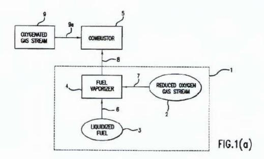
LPP explains that, in the preferred embodiment shown in Fig. 1(a), the fuel gas is produced in a vaporizer unit 4, where the liquid fuel is combined with the reduced oxygen gas stream, producing fuel gas stream 8. See '396 patent at 5:44-50, 6:47-48 ("the reduced oxygen vaporized fuel gas stream 8 is fed..."). This understanding aligns with the Applicant's remarks
