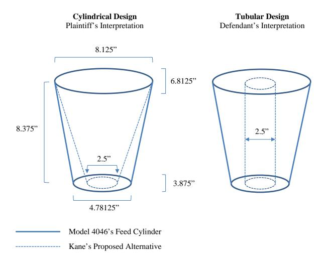
Regardless how Kane's design is interpreted, one thing is evident: Kane would make the bottom of the feed cylinder narrower. As a result, Defendant argues, Kane's design would reduce the Model 4046's feed capacity and thereby reduce its utility to its intended commercial market. Def's MTE at 7–8. In order to claim a product is "defective" in the District of
