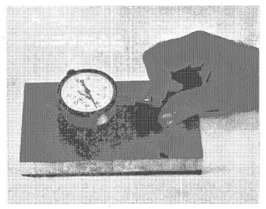
FIG. 16 Lateral Expansion Gage for Charpy Impact Specimens.
