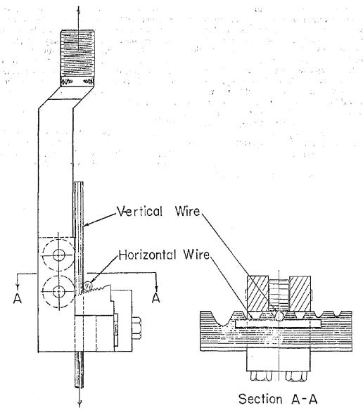
FIG. 1 Welded Wire Fabric Weld Tester.
