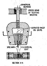
FIG. 38 Wedge-Type Gripping Device.
