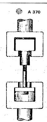
FIG. 33 Tension Testing Full-Size Bolt.
