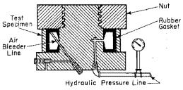
FIG. 24 Testing Machine for Determination of Transverse Yield Strength from Annular Ring Specimens.
