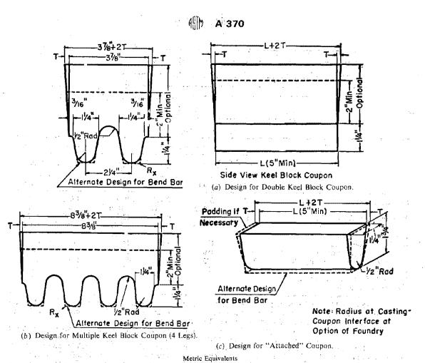
FIG. 3 Test Coupons for Castings (see Table 1 for Details of Design).
