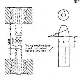
FIG. 18 Metal Plugs for Testing Tubular Specimens, Proper Location of Plugs in Specimen and of Specimen in Heads of Testing Machine.
