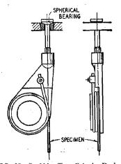
FIG. 39 Snubbing-Type Gripping Device.
