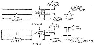
FIG. 11 Simple Beam Impact Test Specimens, Types A and B.
