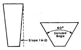
FIG. 30 Tapered Mandrels for Flaring Test.
