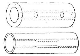
Note.—The edges of the specimen shall be cut parallel to each other.
