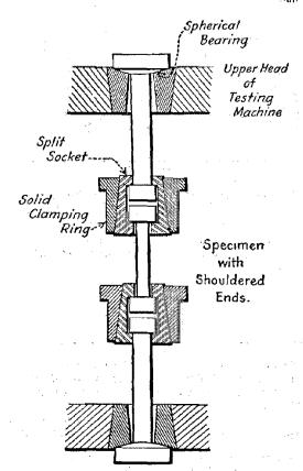
FIG. 3 Gripping Device for Shouldered-End Specimens
