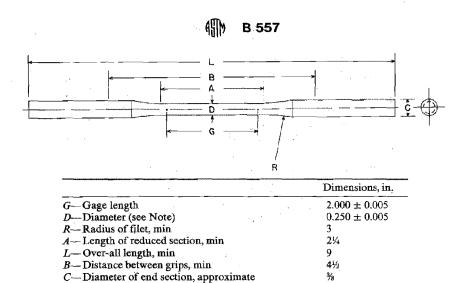
Note—The reduced section may have a gradual taper from the ends toward the center, with the ends not more than 0.005 in larger in diameter than the center.
