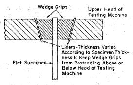
FIG. 1 Wedge Grips with Liners for Flat Specimens
