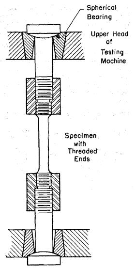
FIG. 2 Gripping Device for Threaded-End Specimens
