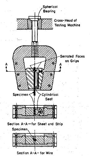
FIG. 4 Gripping Devices for Sheet and Wire Specimens
