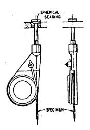
FIG. 5 Snubbing Device for Testing Wire
