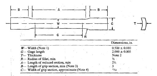
NOTE 1—The ends of the reduced section shall not differ in width by more than 0.002 in. There may be a gradual taper in width from the ends of the reduced section to the center, but the width at each end shall not be more than 1 % greater than the width at the center.
