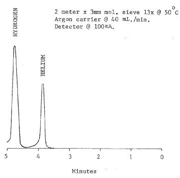
FIG. 8 Separation of Helium and Hydrogen
