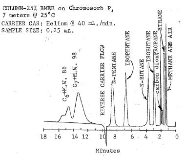
FIG. 4 Chromatogram of Natural Gas (BMEE Column) (See Annex A2)
