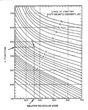
FIG. 1 Viscosity-Molecular Weight Chart
