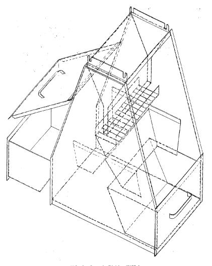
FIG. 3 Sample Divider (Riffle)
