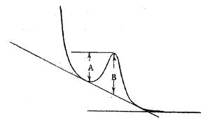
FIG. 2 illustration of A/B Ratio for Small-Component Peak
