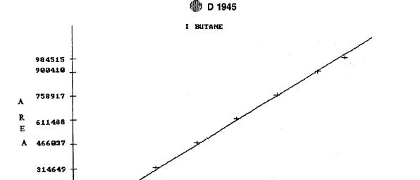
FIG. X1.1 Example of Deriving a Relative Molar Response Factor
