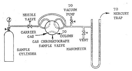
FIG. 1 Suggested Manifold Arrangement for Entering Vacuum Samples
