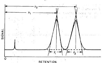
FIG. 2 Calculation for Resolution
