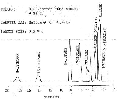
FIG. 6 Chromatogram of Natural Gas (See Annex A2)
