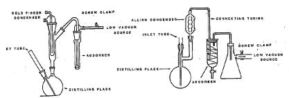
FIG. 1 Cyanide Distillation Apparatus
