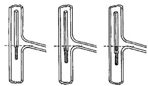
FIG. 5 Position of Thermometer in Distillation Flask
