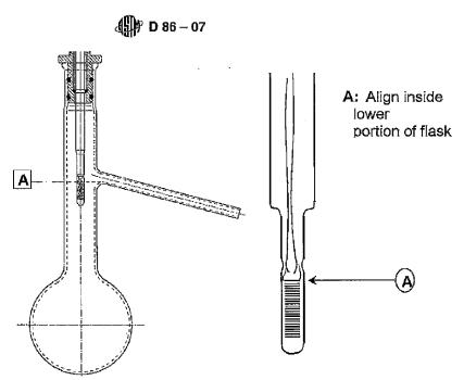
FIG. 6 Example of Recommended Placement of Pt-100 Probe Relative to Distillation Flask Sidearm for Automated D 86 Distillation Instrument
