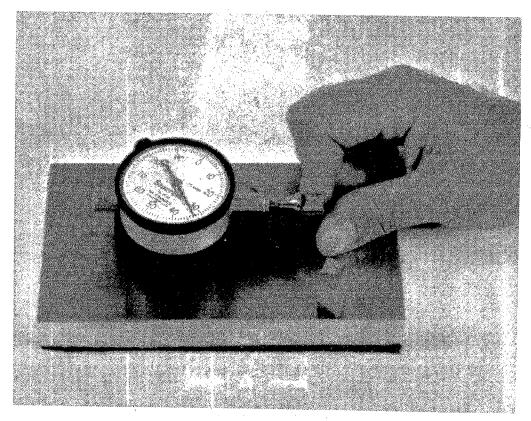
FIG. 17 Lateral Expansion Gage for Charpy Impact Specimens
