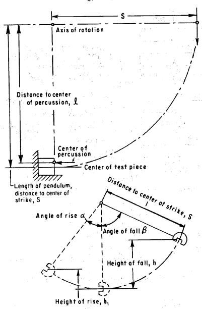
FIG. 5 Dimensions for Calculations
