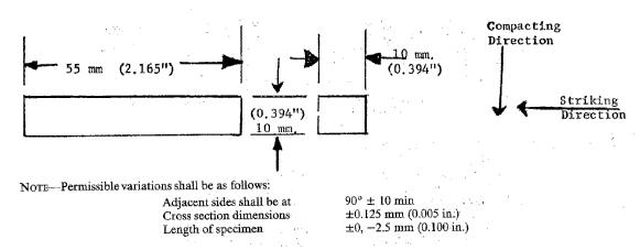
FIG. 9 Charpy (Simple Beam) Impact Test Specimens for Metal Powder Structural Parts
