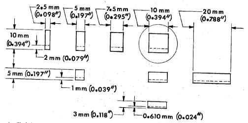
NOTE 1—Circled specimen is the standard specimen (see Fig. 6).
