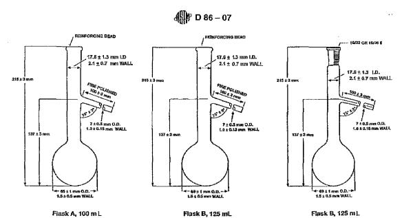
FIG. A2.1 Flask A, 100 mL, Flask B, 125 mL, and Flask B with Ground Glass Joint, 125 mL
