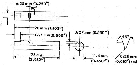
The flat shall be parallel to the longitudinal centerline of the specimen and shall be parallel to the bottom of the notch within 2:1000.
