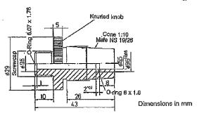
FIG. 3 PTFE Centering Device for Ground Glass Joint
