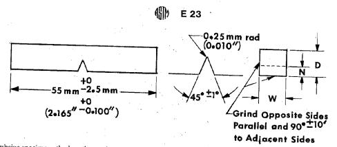
On subsize specimens the length, notch angle, and notch radius are constant (see Fig. 6); depth (D), notch depth (N), and width (W) vary as indicated below.
