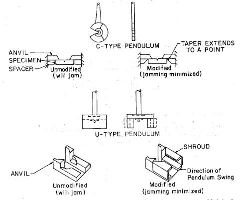
FIG. 1 Typical Pendulums and Anvils for Charpy Machines, Shown with Modifications to Minimize Jamming
