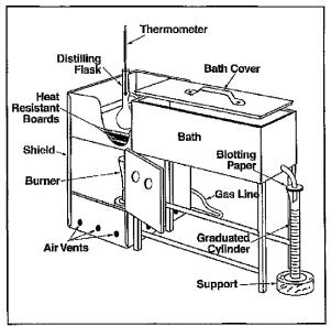
FIG. 1 Apparatus Assembly Using Gas Burner
