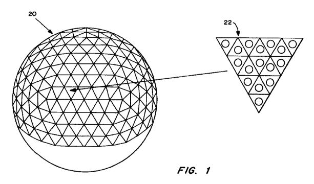
'134 Patent Fig. 1, 4:46-52 ("FIG. 1 is an exploded view showing a phased array antenna of the present invention which comprises substantially equilateral triangular-shaped subarrays of antenna elements mounted on the faces of a geodesic sphere structure with one of the triangular subarrays broken away and enlarged for purposes of illustration . . . .").
