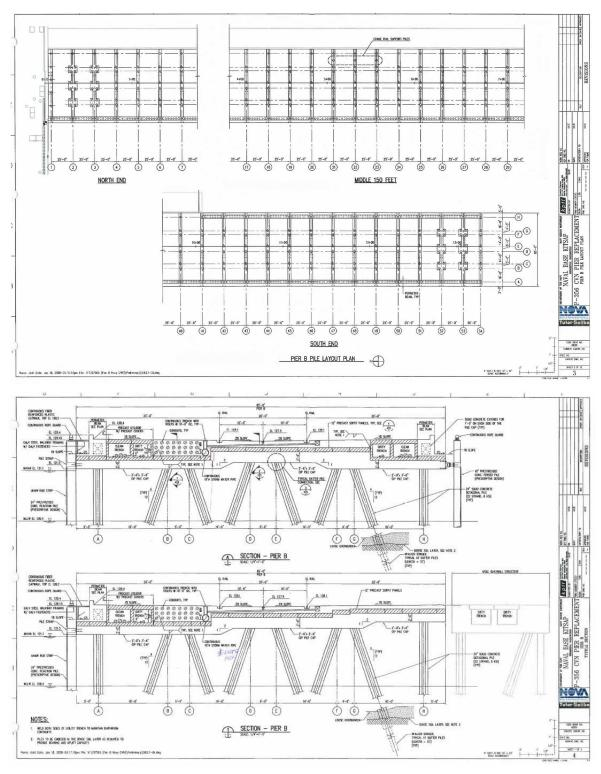
JX 4.211-12. Pier B piles in Rows A and H, as well as all piles in Bent 1, were designed as vertical (or plumb) piles. <u>Id.</u>; JX 50.1-.5; JX 53. Pier B piles in Rows B, C, D, E, F, and G were designed
