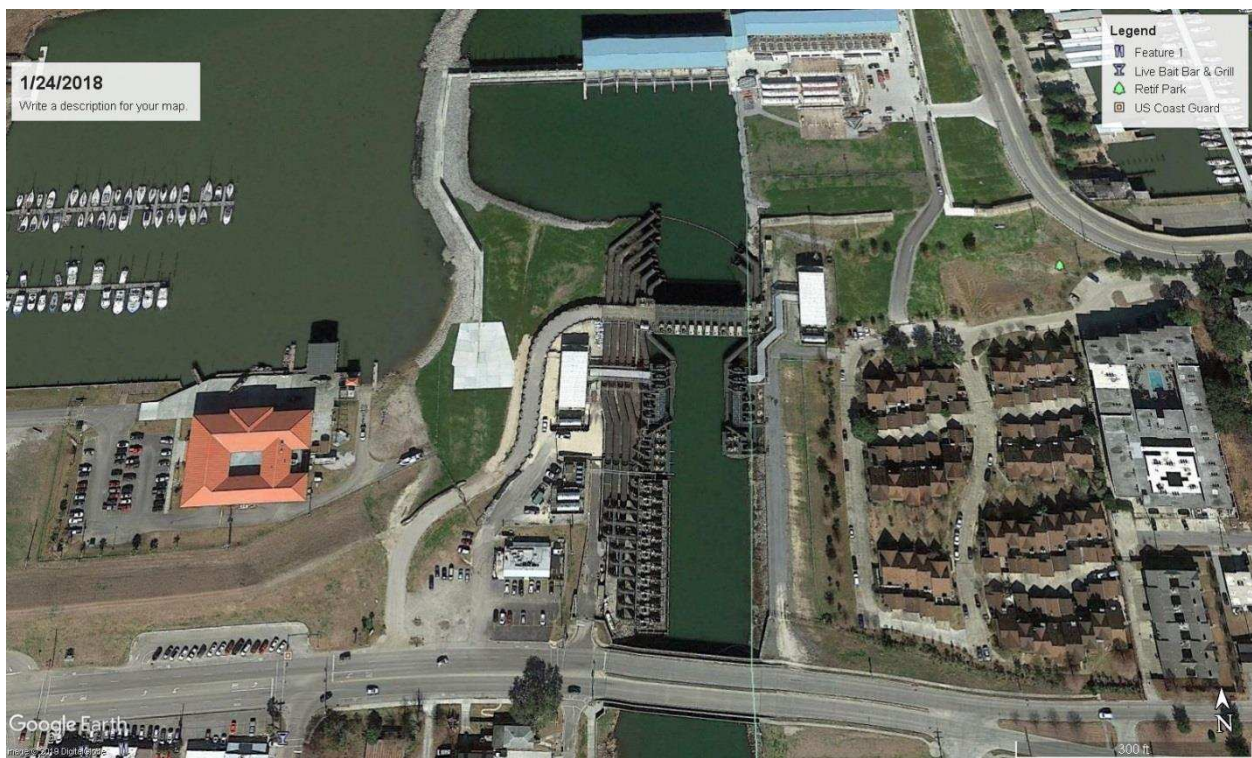
Figure 3: Satellite Imagery of Figure 1 advanced to January 24, 2018. A new closure structure, basin, and levee walls appear. Imagery from 2019 appears to show that removal of the interim pump station and related structures has commenced.
