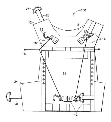
An individual has pulled on the pull cord (16) appearing on the left side of the figure. As a result, the left cord (18) has been tightened, causing the two releasable hooks (13) to disengage. The right pull cord (16) has not been pulled, so the right releasable hooks (13) remain engaged.
