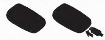
The two Charging will be visible on the screen when your Neonode is properly connected and charging. This taxt will show as long as the device is connected to the charger/computer. Your Neonode can be charged either turned on or off. If it is turned off, you have to disconnect your Neonode from the USB cable when finished charging before you can turn it back on.
