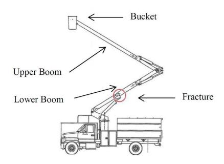
On April 9, 2014, Plaintiff Jeffrey Gaddy ("Plaintiff") was in the bucket of the Subject Boom Truck when the lower boom stub fractured, causing Plaintiff to fall to the ground. Plaintiff suffered spinal injuries resulting in paraplegia.
