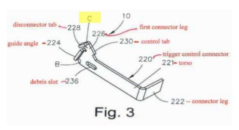
According to Lone Wolf, the 342's "third predetermined angle ("C")" is ninety-seven (97) degrees and because 97 degrees does not fall within the 81 to 91-degree range as required in the '700 patent, the 342 is not an infringing product. Conversely, Patent Holder alleges that the third predetermined angle of the 342 device is actually 89 degrees and does fall within the '700 patent.
