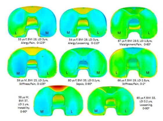
"colormetric maps of deformation" in the polyethylene surface:
