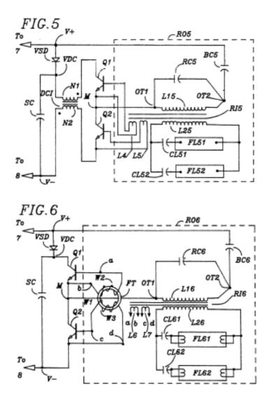
(*Id.* at Figs. 5, 6.) Finally, the patent explains that the circuit in Figure 5 "is identical in operation to the one [in] FIG. 1, with the exception that the resonant elements"—*i.e.*, the resonant capacitor and the resonant inductor—"are connected here in parallel." (*Id.* at col. 9,
