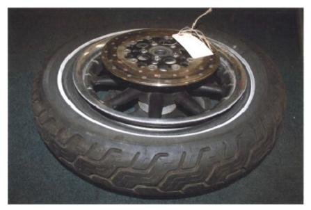
The Timms' theory of the defect in this case is that there was excess "flash" in the bead area and too thin rubber covering the chafer strip which, in combination with the rim, resulted in an insufficient amount of rubber in the bead area, weakening the
