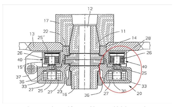
In this image, molten metal flows out of the opening labeled No. 12. The opening is closed off at various points by the refractory plates, labeled Nos. 22 and 23.
