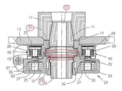
The slide gate operates so that rollers (No. 27) roll along a track (No. 36), such that in this image, the slider unit (No. 30) would roll on a track towards you or away from you. This action either opens or closes the refractory valve plates, allowing liquid metal to flow out of the opening (No. 12) or keeping it inside of the container, depending on whether the plate is opened or closed.
