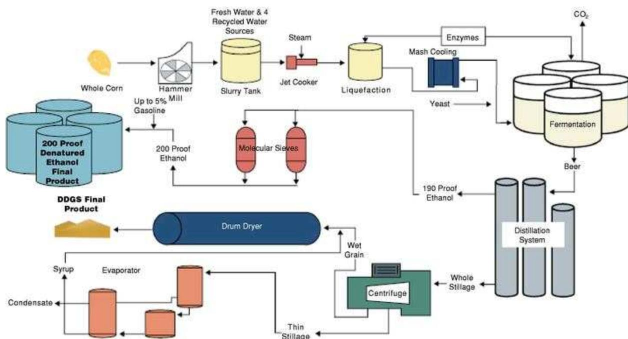
Starting in the upper right-hand corner of the diagram, the process begins with the corn being ground into meal and then mixed with hot water, recycled thin stillage, and enzymes. MDN 1173 at 16. The mixture is heated or “cooked” to form a less viscous, liquefied “mash” stream. *Id.* The mash stream is then fermented with yeast to produce
