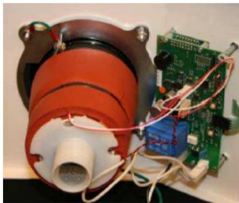
The above-picture shows what a user would see after opening the warmer. Doc. 119-2 at 10–11, ¶ 28. An orange foam insulation blanket covers the exterior of the cup. Mr. Koch asserts that he followed the teachings of the '498 Patent when he designed the warmers and used a synthetic cork insulative material formed from a piece of silicone sheet. Mr. Koch also designed the warmers with an insulative material that is molded to a desired shape by wrapping the
