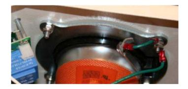
Doc. 119-2 at 16, ¶ 42. The zip-tie secures the damper to the exterior surface of the cup so that the damper can reduce relative movement of the cup in relation to the cover when the vibration function of the warmer is activated. If a user removed the damper zip-tie, the user would have to supply a new zip-tie to reattach the damper to the exterior surface of the cup.
