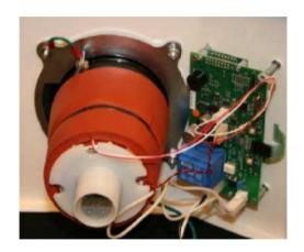
The above-picture shows what a user would see after opening the warmer. Doc. 119-2 at 10–11, ¶ 28. An orange foam insulation blanket covers the exterior of the cup. Mr. Koch asserts that he followed the teachings of the '498 Patent when he designed the warmers and used a synthetic cork insulative material formed from a piece of silicone sheet. Mr. Koch also designed the warmers with an insulative material that is molded to a desired shape by wrapping the
