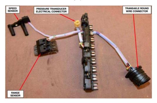
This specific wire harness is used to carry signals which determine when the automatic transmission needs to shift. The wire harness plugs into the valve body assembly—essentially
