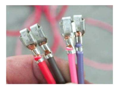
Large-scale manufacturing assembly plants, like the ones used by ZF NA and FCA US, make crimps by using automated machinery with specific crimp specifications. The wiring crimp then allows the wire harness to be "plugged into" the appropriate connector for whatever purpose it is being used, as displayed in the following picture.<sup>9</sup>
