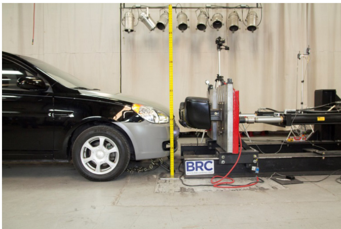
Figure 2. Photograph of the test apparatus modified for an override/underride condition. The fixed steel plate has been removed and a whole vehicle is rigidly anchored to the ground and fixture.
