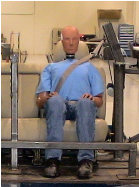
Figure 2 Photograph demonstrating the occupant, seat, and restraint configurations used in sled tests.
