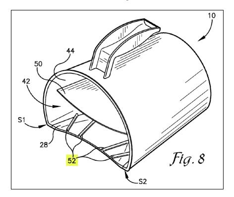
'178 Patent at Figure 8 (highlight added). The specification states that "ridges 52 are, in a preferred embodiment, molded of the same material which flexible panel 28 is constructed ... however, it is desirable that ridges 52 do not obstruct the flexibility of panel 28 as it should be readily
