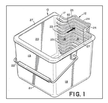
[Doc. No. 406-6 at Figure 1]. As shown in Fig. 1 of the Perock Patent, the inner surface of the flexible panel area 17 includes a series of corrugations (23).<sup>7</sup>
