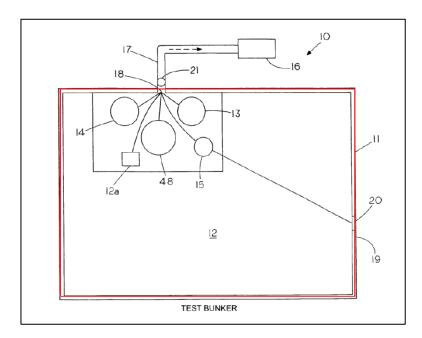
*Id.* at Figure 1 (annotated). The specification states that the high pressure testing equipment (*i.e.*, low-pressure pump 13, intermediate-pressure pump 14, high-pressure pump 48, and bleed valve 15) are enclosed in housing 11. *Id.* at 3:13–16. Similarly, in describing an alternate embodiment, the specification states that "unlike the bunker housing 11 of safety system 10, which comprises a
