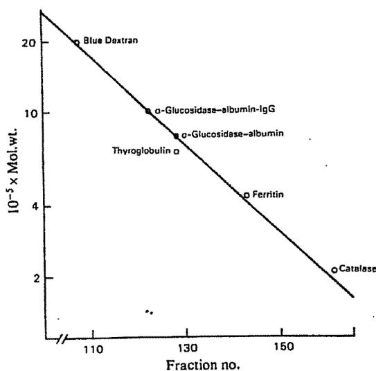
FIG. 1. Molecular weight determined of  $\alpha$ -1,4-glucosidase-albumin polymers. Gel chromatography was employed using Bio-Gel A-50M with Pharmacia standards; catalase, ferritin, thyroglobulin and blue dextran 2000. Over 80% of the enzyme-albumin polymer eluted between peaks 124 and 132 indicating a MW range of  $7.5 \times 10^5$  to  $9.5 \times 10^5$ . The addition of anti-hepatocyte antibodies to the polymer resulted in an average increase in MW of  $2 \times 10^5$ .
