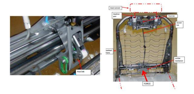
But Lear seeks leave to "identif[y] an alternative four-bar mechanism" on the accused device. (ECF No. 54-8, PageID.5498.) In particular, Lear seeks to amend its infringement contentions to identify different first, second, and third links of the four-bar mechanism on NHK's device:
