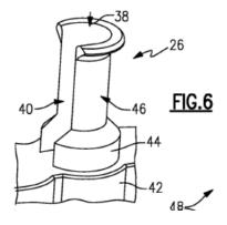
('420 patent Fig. 6.) This drawing, along with the description of a pin bar as an "integral structure having... pins," especially when contrasted against the disclosure regarding detachable pin bars and bases, would lead a person having ordinary skill in the art to conclude that the phrase, "a base; and a plurality of pins supported on the base" to encompass an integrated pin-base design.
