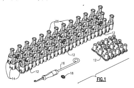
('565 patent Fig. 1.) In an embodiment of Choon's invention, openings (30) in the bottom of the pin bar (14) fit snugly over cylinders (28) of a base (12) so that the pin bar ends up mounted on the base:
