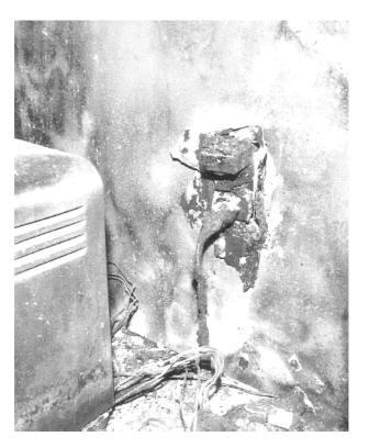
(Pls.' Resp. to Def.'s Mot. Summ. J. Ex. A.) The Black & Decker charger is plugged into the top receptacle and a power strip is plugged into the bottom one.
