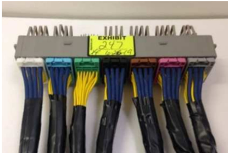
Figure 3: Wire Harness for GM's BCM Connected to HIT2
