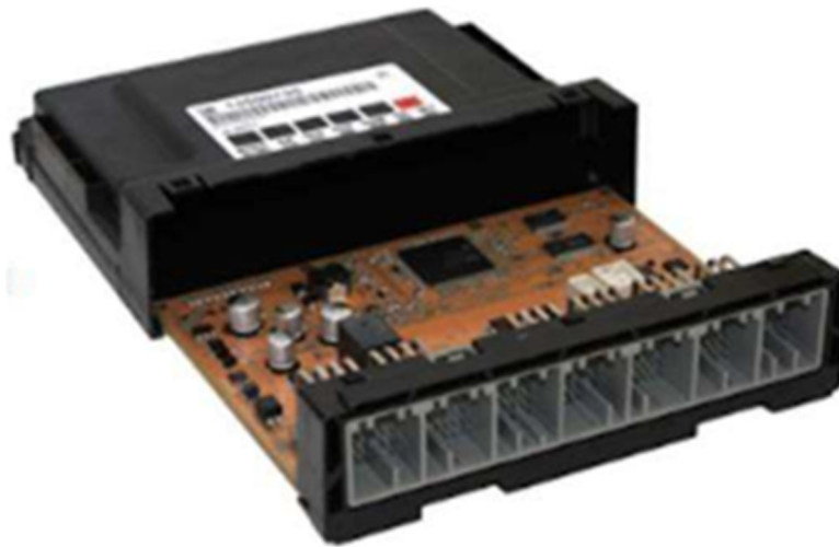
Figure 2: HIT2 within a GM Body Control Module ("BCM") Assembled by Bosch
