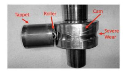
(PageID.821.) The limited contact area between the cam and roller, the high force at the contact area, the roller and cam's lubrication sensitivity, and the possibility of the tappet rotating out of position together contribute to an allegedly "fragile" design.
