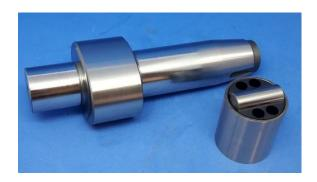
Cam-Shafts & Rollers of CP4 Pump, Sirini, https://perma.cc/63K9-PECZ. The CP4 pump has a pair of roller-tappet systems that operate identically. (See PageID.814.) In operation, the oval-shaped cam spins, and the battery-shaped roller rolls along the cam. (See PageID.814.) The picture below shows how the cam's rotation moves the tappet up and down and thus pumps fuel (on the left, the cam has pushed the tappet to the high position, while the tappet on the right is in the low position).
