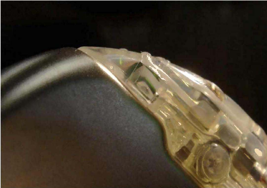
Figure 1. Photograph showing the DF- wire in the Braund device. No cracking is evident in the wire insulation, the point of maximum bend is not in contact with the backfill tube, and MA filled space exists between the backfill tube and the DF- wire insulation.
