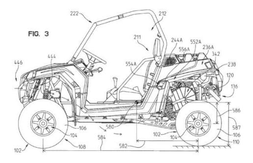
('501 Patent at 52.) The specification then provides that the "center of gravity **580** of an **unloaded vehicle**... is positioned a distance **582** forward of rear axle... and a distance ... above the rear axle... Center of gravity **580** is generally centered close to or on vertical centerline plane" of the vehicle. (*Id.* at 109-10 (emphasis added).)
