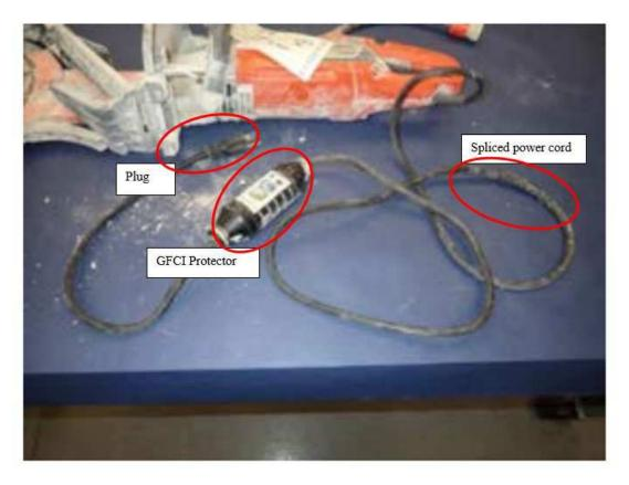
[Doc. 53-7 at 21] (19-180-154.jpg, annotations added). Because Reagan found the GFCI device to function properly, it presumably would have cut off the flow of electricity were
