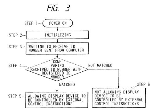
This flowchart clearly shows one use of an identification number *sent by the computer*:<sup>5</sup> it is received by the microcomputer in the display device, which checks to see if the number is registered, and then the outcome of that check determines whether or not the computer will be
