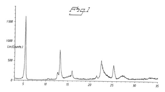
The diffractogram of Figure 1 shows position (x axis) plotted against intensity (y axis), obtained when a powder sample is irradiated with X-rays at various angles indicated by the values on the x axis.
