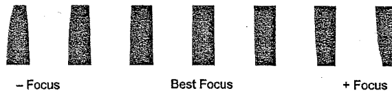
Figure 3.11 Variation of the resist profile shape through focus in the presence of coma
